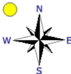
Fig. 6 a Hillshade's sun's default azimuth (direction) is 315° (Source Esri ArcMap 10.3)
